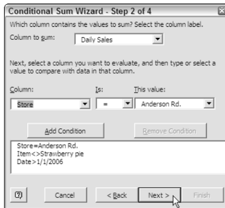
Figure 9-4: The Step 2 of 4 Conditional Sum Wizard dialog box after speci- fying the column to sum and the conditions to use.
